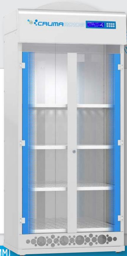
**Cruma 2010 vented chemical storage cupboard**, with the same filtration technology used by Cruma in its fume cupboards during more than 30 years, allow the storage of liquid reactives, reducing the space used, and removing the inflammable, corrosive or toxic vapours by adsorption by means of an specific activated carbon filter, and recirculating the purified air into the laboratory.
