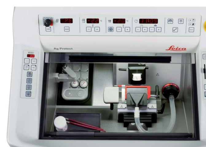
Efficient specimen loading is achieved via single lever operation that provides maximum clamping force independent of individual user strength.Direct contact cooling through the (optional) actively cooled object head facilitates rapid changes of specimen temperatures to provide the best conditions for sectioning various specimen types.
