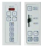
Easy for the multi users: the selfexplanatory, single-function keys and easily readable LEDs help prevent operating errors, facilitate cryosectioning, and make scrolling through multiple menus unnecessary. The control panels are comfortably positioned in the armrests to eliminate the need to reach into the cold chamber to use or adjust settings.
