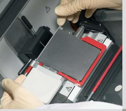
The new disposable blade holder CE with integrated, colored safety guard and blade removal aid makes blade handling safer. For users who prefer using the brush technique during sectioning, the palm rest can be used instead of the anti-roll guide.
