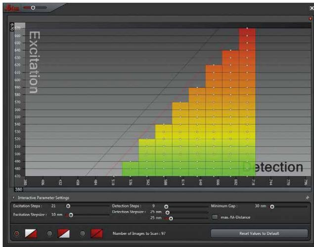
User interface for spectral excitation-emission FCS or FLIM scan. Find the optimal setting for your dye.
